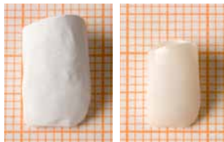
Fig. 37: The oversized preform made of zirconium oxide (Lava™, 3M Espe) in milled and unsintered condition and the sintered crown framework.
